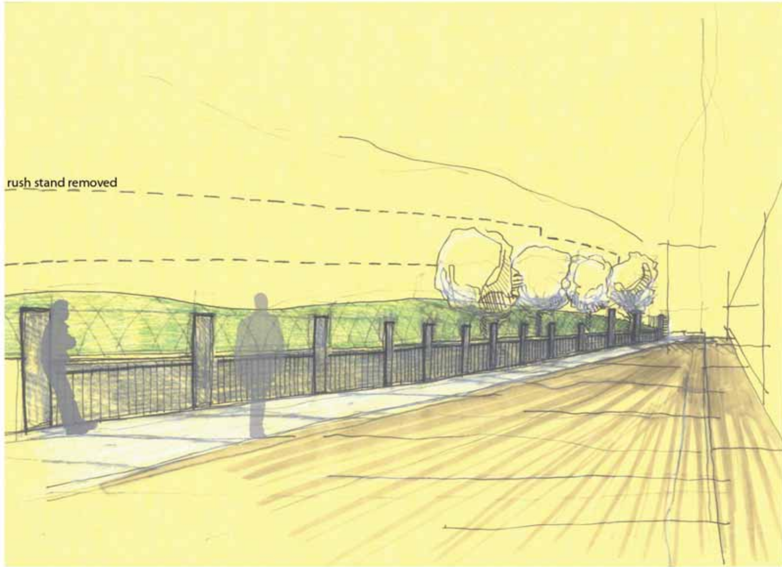
view 3 view looking east along turner street. rush stand removed. perimeter fencing reduced to 1.2-1.5m high
